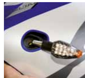
Etape 2 : Placer le cache-orifice. Place the blanking light.
