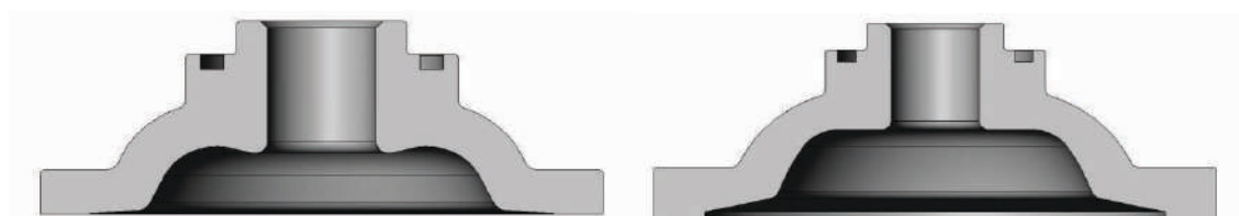
Fig. 1 Example custom insert with different shape of combustion chamber
